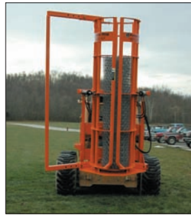
Fast job setup! The Fence Hog picks up a roll of chain link and within minutes you're ready to stretch it to the posts.
