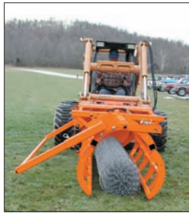
Fast job setup! The Fence Hog picks up a roll of chain link and within minutes you're ready to stretch it to the posts.
