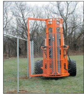
Fast job setup! The Fence Hog picks up a roll of chain link and within minutes you're ready to stretch it to the posts.
