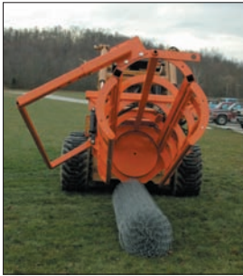
Fast job setup! The Fence Hog picks up a roll of chain link and within minutes you're ready to stretch it to the posts.
