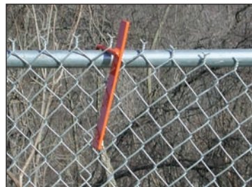
The Hog Stringer dispenses bottom tension wire with ease, while the Hog Hangers slide easily on the top rail to temporarily hold the fence.
